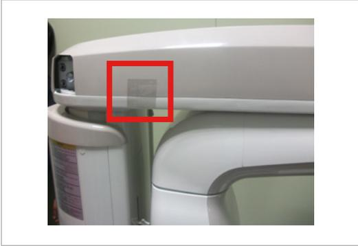
1. Remove the semi-clear tape on both sides and open the top cover.
