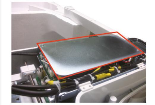
1. Remove the 4 screws to separate the top cover.
