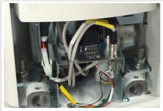
6. Arrange the cable carefully and if necessary, tie them with the cable tie (Part No.10)
