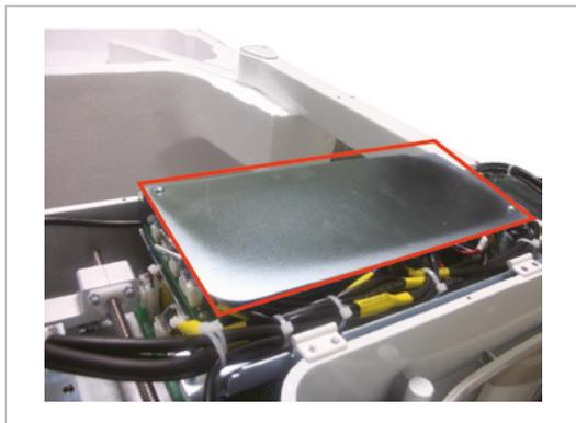
1. Remove the 4 screws to separate the top cover.
