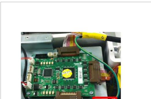
5. Connect the ground cable (FG) to the frame.
