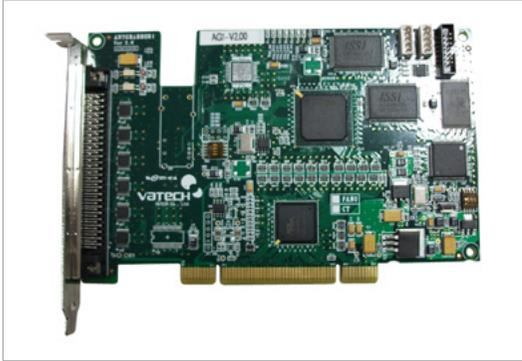
4. Insert the frame grabber board: AnyGrabber board (**Part No.27**) firmly into that slot.
